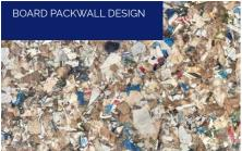
The beginning of the whole process lies in the collection of beverage cartons with the lowest content of things that have been mistakenly put in the orange containers for sorted waste – glass, wood, metal, etc. beverage cartons are subsequently crushed, dried, moulded under high temperature into the boards and cut into appropriate formats. The boards are basically a composite composed of cellulose, polyethylene and aluminium (all components of food cartons) enclosed between two paper surfaces.
